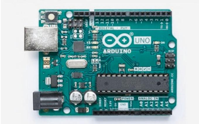
**Fig. 1** Microcontroller unit based on ATmega328 microcontroller – Arduino Uno R3
