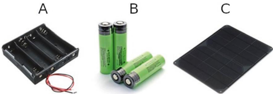
**Fig. 5** The power supply of the system: (a) the battery pack, (b) 18,650 batteries, and (c) solar panel
