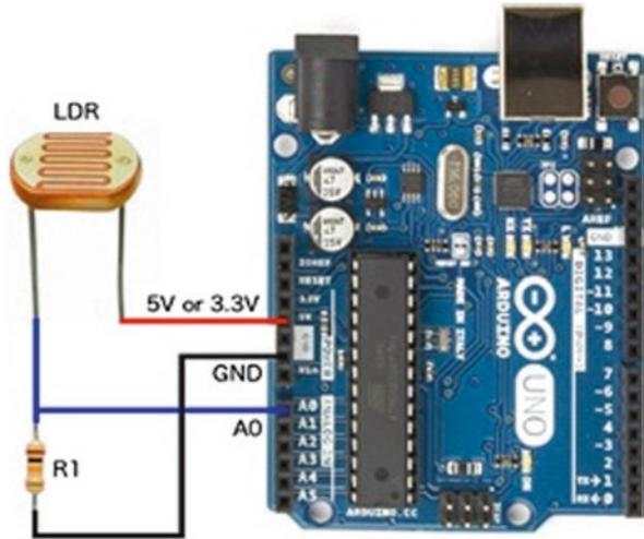
The sensor is powered directly from the microcontroller board due to its operational power supply range (3.3 V or 5 V) and its power dissipation which is very low.
